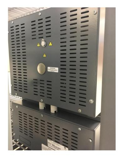
The back of the furnace should look something like this. Remove the thermocouple by unscrewing the flange holding it in place in the top portion, and then unscrew the wires from the electrical components before passing said wires through the plastic bushings, and removing the thermocouple entirely.
