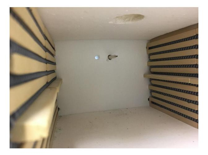
Screw the flange back into place on the thermocouple's lower ceramic covering, and the furnace should be operational. If the proper chromel/alumel thermocouple is used (Part # TC1165X1), no calibration should be necessary. Plug in the furnace and turn it on to make sure it is functional.
